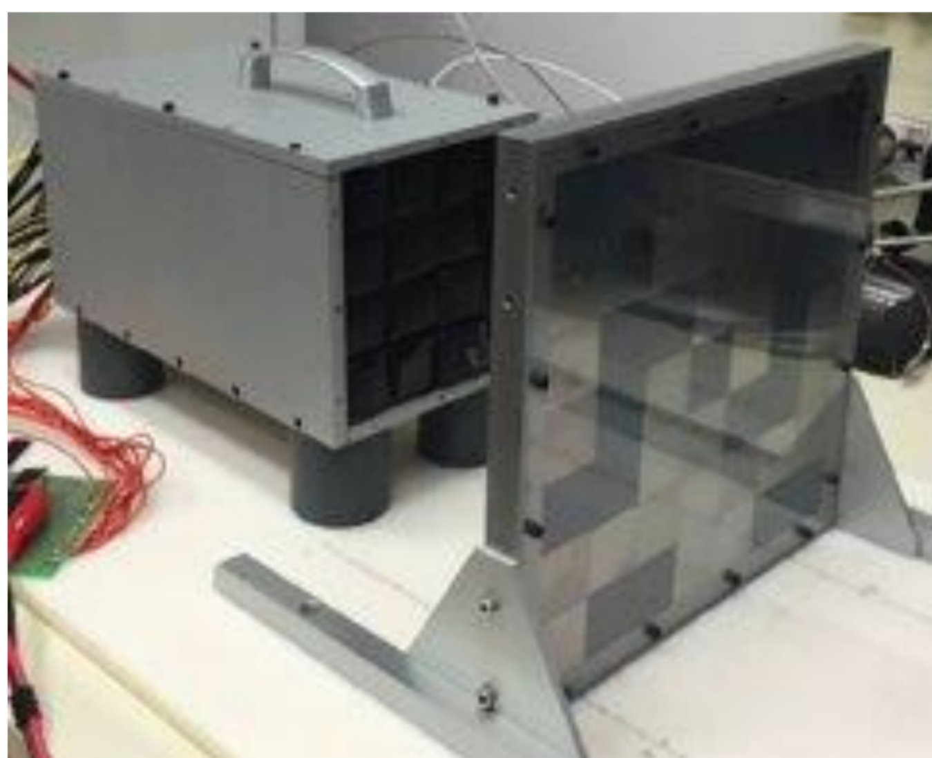
Fig. 4. the HERGA prototype, shown as an example of integration of CAEN electronics for Gamma-rays monitoring.
