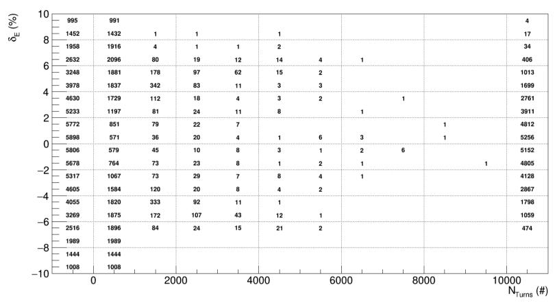
Tracking has been performed with PTC (MAD-X interface) for **10k turns**. Initial distribution are Gaussian with **nominal emittance** (CDR  $\varepsilon_x$ :1.29  $\varepsilon_y$ :1.22 10<sup>-6</sup>m rad). Tracking includes **radiation loss** and **RF effects**.
