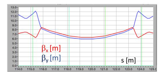
Ideal section no SXT Injection Kickers position optimized Twiss function are not optimal for injection
