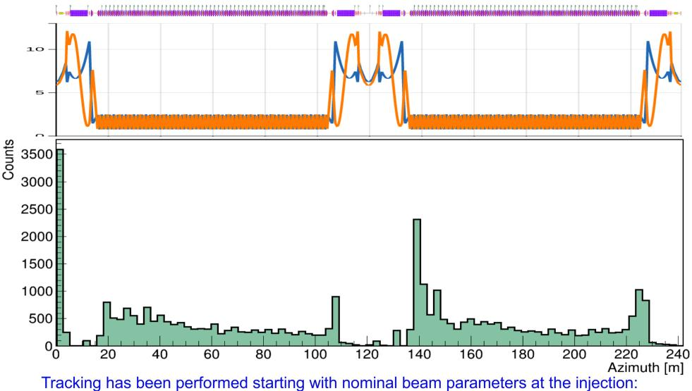
Gaussian profile with nominal width ( $\sigma \sim 2$ mm in both planes). The energy distribution has been assumed Gaussian with 5% resolution.
