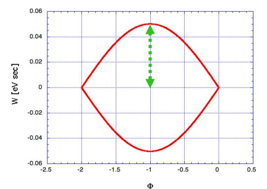
$$\frac{1}{\Omega_s} \frac{d\varphi}{dt} = \frac{2\pi c}{L} \sqrt{\frac{2\pi h^3 \eta_{tr}}{E_s eV \cos \varphi_s}} W$$
