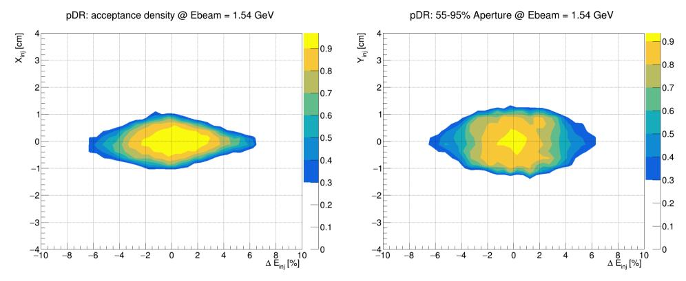
DR acceptance probability has been evaluated starting with nominal beam parameters at the injection: Gaussian profile with nominal width at the injections ( $\sigma \sim 2$ mm in both planes). The energy distribution has been assumed Gaussian with 5% resolution.
