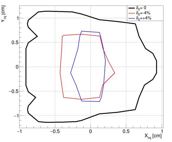
2000 turns have been tracked (~15% damping time). The estimated loss of accuracy is below 1% at the nominal energy.
