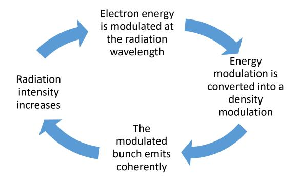
There is an energy-transfer between the electrons and the radiation field. Internal micro-bunches appear in the electron bunch at the radiation wavelength. Each micro-bunch effectively acts as a point-source, emitting coherent radiation proportional to the square of the number of electrons within that segment.
