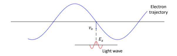
As the electrons travel along the undulator, the radiation slips forward ahead of the electrons. In order for there to be sustained energy transfer from the electron beam to the light wave, the light wave must advance by  $\lambda_r/2$  when the electrons have travelled a distance  $\lambda_u/2$ .
