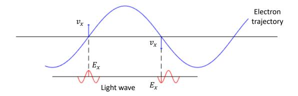
This is the same condition as for constructive interference in an undulator, i.e. the condition for continuous energy transfer from the electron beam to the light wave is:
