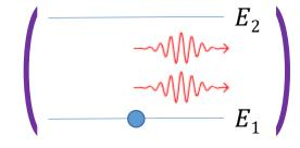
1) Gain medium is put into an excited state by the energy pump (population inversion) 2) Incident photon at the energy  $\hbar \omega = E_2 - E_1$ increases the likelihood of electron transition to the lower energy state 3) As the atom changes state it emits a photon of energy  $\hbar\omega$
