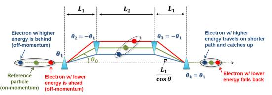
**Fig. 2**: Geometry (not to scale) of a four-dipole symmetric magnetic chicane, and particles' motion through it for the case of bunch-length compression. See context for the meaning of symbols.
