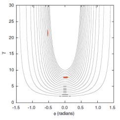
**Fig. 7:** Phase-space apparent rotation in RF sinusoidal accelerating field, leading to bunch-length shortening for a bunch injected near the phase of zero crossing. Published in Ref. [29]. Copyright of American Physical Society.
