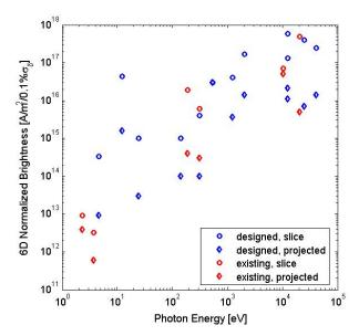
**Fig. 1**: 6D normalized electron-beam brightness (Eq. (1)) vs. maximum photon energy at fundamental FEL emission, for facilities in the UV to X-rays, in design stage (blue) or operational (red), up to 2013. From lower to higher photon energies, "existing" facilities are: SPARC (Italy), SDUV-FEL (China), FLASH-I (Germany), FERMI (Italy), LCLS (USA), SACLA (Japan). The brightness refers to the projected (circle) or slice value in the bunch (diamond). Published in Ref. [2]. Copyright of Elsevier.
