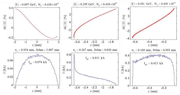
**Fig. 4:** Longitudinal phase space (top row) and current profile (bottom row) of a 700 pC charge bunch injected into the S-band FERMI FEL linac at 97 MeV (left). Centre plots are for the beam after magnetic compression in a four-dipole chicane, with no linearizer included. Right-hand plots are for the same beam when an X-band cavity in the upstream linac is set to -15 MV, for linearization of the compression process. Simulations were done with LiTrack code and up to second order.
