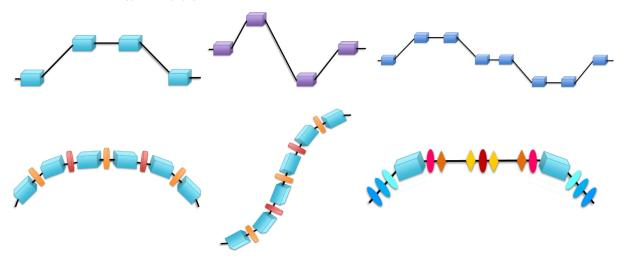
**Fig. 6:** Most common geometries (not to scale) of magnetic insertions for bunch-length compression. From top, left to right: C-shape, S-shape and double C-shape chicanes; bottom, arc-fodo, dog-leg-fodo and double-bend achromatic cells.
