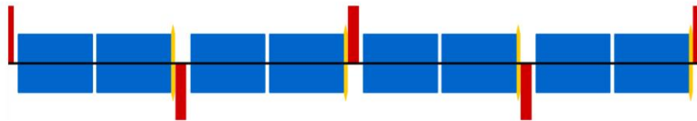
Fig. 6: Schematic of an interleaved sextupole scheme for a FODO cell lattice with \varphi = 90^\circ phase advance in both planes. After every quadrupole a sextupole magnet is installed leading to a maximum number of sextupoles. The sextupoles that are separated by a phase advance of \pi form a family. In this case there are two families per planes.
