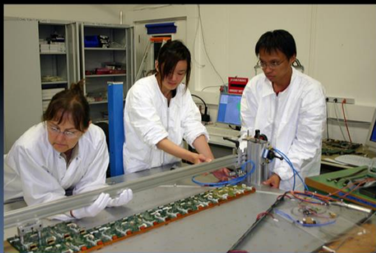
Testing a column of ladders
