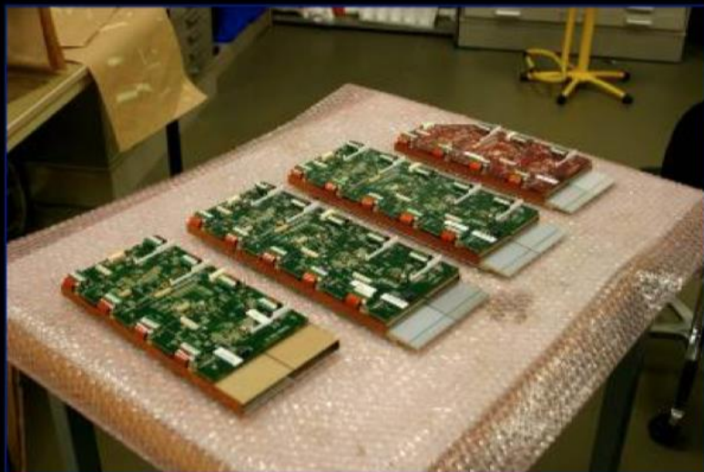
3 types of "ladder" filled with Si sensors
