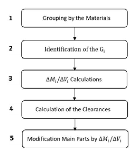
The purpose is to compensate for material loss after the  $\Pi_1$  and keep mass properties and volume of the initial, non-simplified geometry
