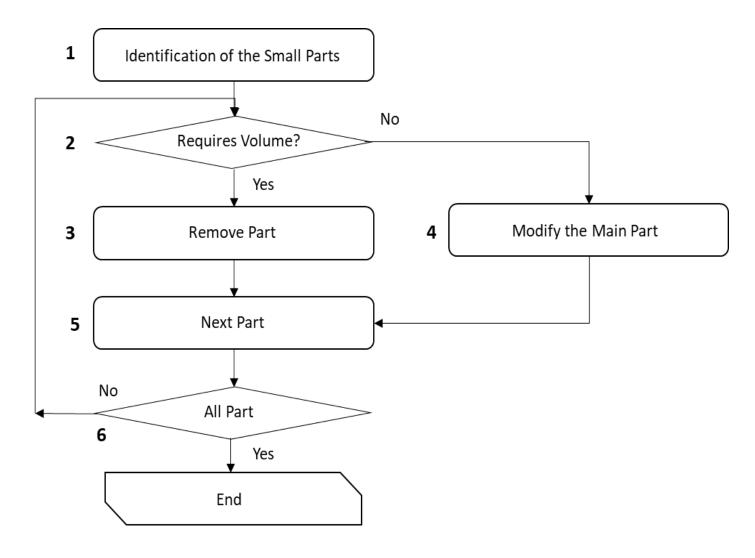
The number of volumes in the geometry is the key factor - as many volumes are described in the geometry, the simulation performance is less.
