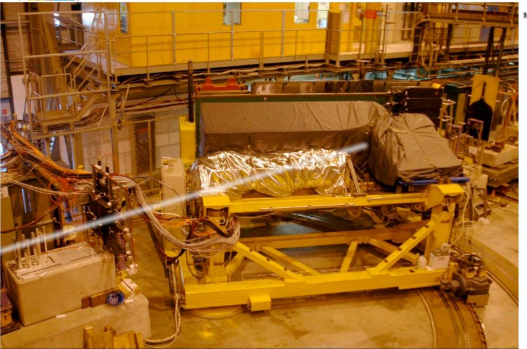
This test beam setup provided measurements of energy response and energy resolution for pi-plus, kaons of either charge, antiprotons of momenta between 2 and 9 GeV, pi-minus of momenta between 2 and 300 GeV and protons of momenta between 2 and 350 GeV
