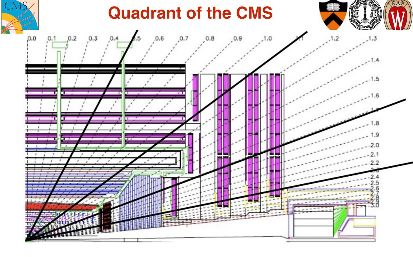
Four partitions in the CMS detector are used in the measurement of calorimeter response
