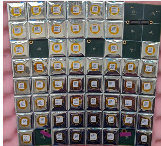
TB3 board 2 equipped with moulded tiles Batch 2 with pre-series 4mm 2 SiPMs
