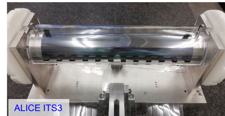
Bent wafer-scale dummy sensor on foam support
