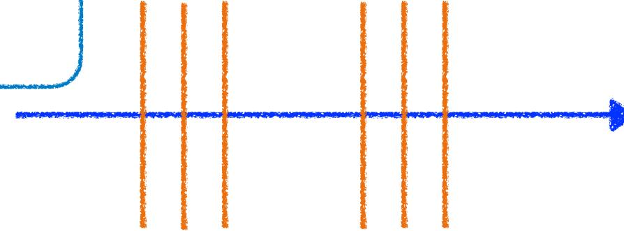
Beam 6 layer telescope Trigger scintillators
