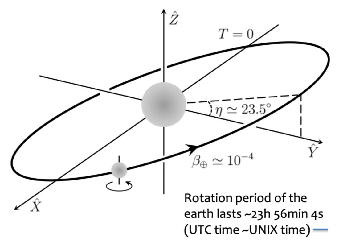
CMS frame is rotating around the earth Z-axis → modulation of the top-anti top cross section with sidereal time
