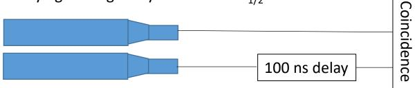
Due to the delay, the coincidence will not see the muons signals any longer at the same time (i.e. within the coincidence window) and the muons "disappear". The noise, however, will not notice the delay due to its random nature
