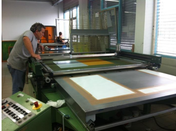
Semi automatic screen printing machine Printing area 2m x 0.9m for posters (Satigny)
