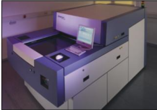
Figure 2 e 3 – The Paragon-8000 Laser Direct Imaging system (above) and 25 \mu\text{m} features exposed using this system (below)
