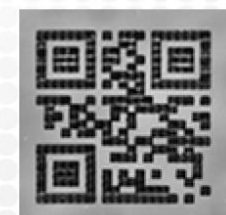
Micro QRcode (750 μm × 750 μm)
