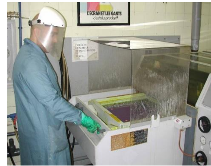
Copper Etching Chemical spray
