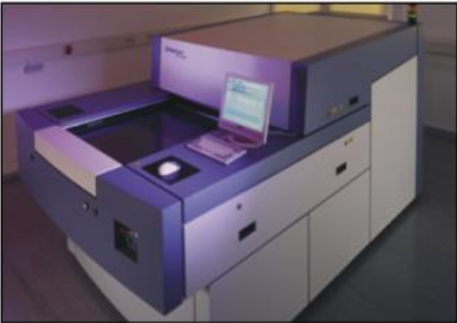
Figure 2 e 3 – The Paragon-8000 Laser Direct Imaging system (above) and 25 \mu m features exposed using this system (below)
