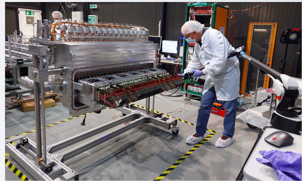
Laser metrology, before installation
