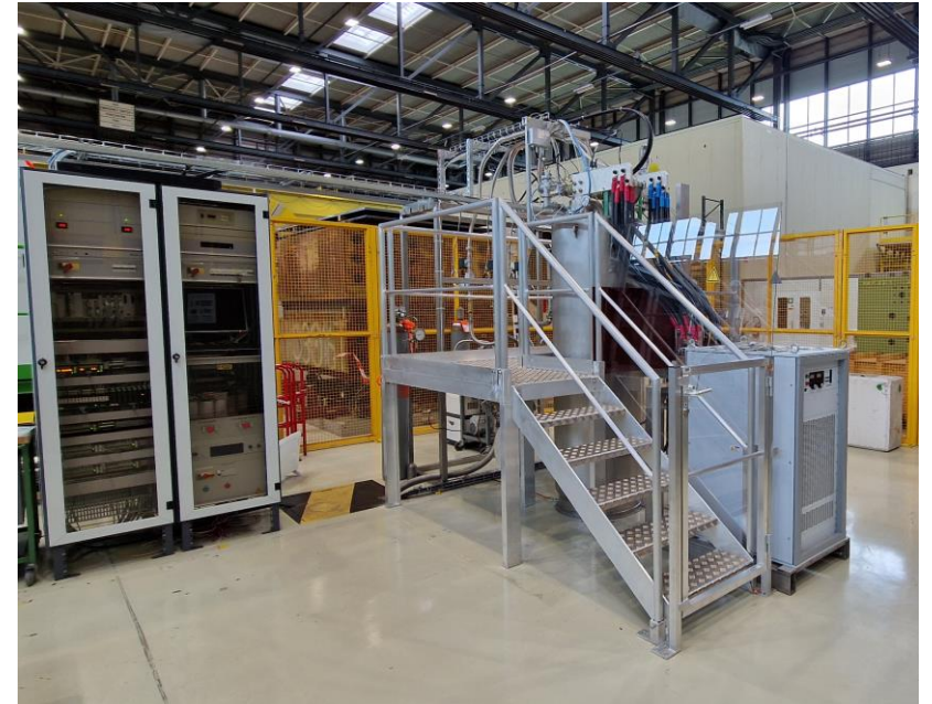
Cryogenic test station featuring 5 T solenoid
