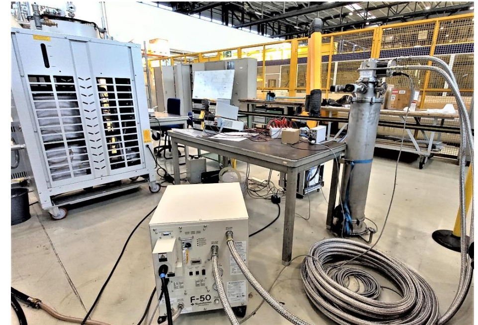
Test set up for cryo-cooler performance check in b180
