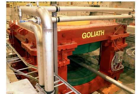
Goliath normal-conducting dipole
