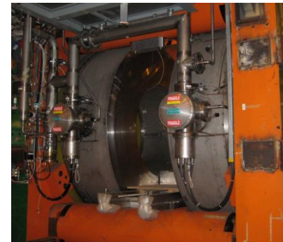
M1 superconducting dipole
