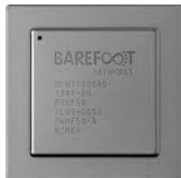
Figure: Intel Tofino P4-programmable Ethernet Switch ASIC
