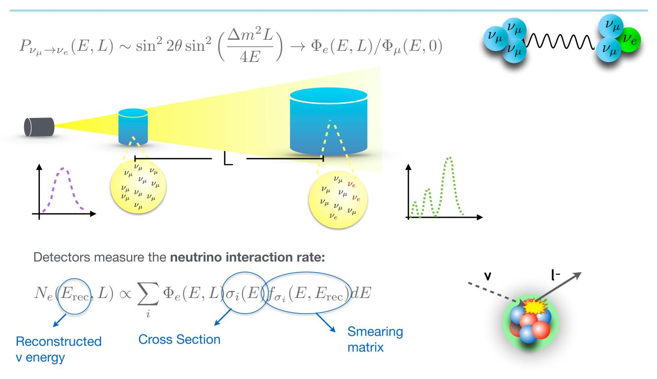
A precise determination of  $\sigma(E)$  is crucial to extract v oscillation parameters
