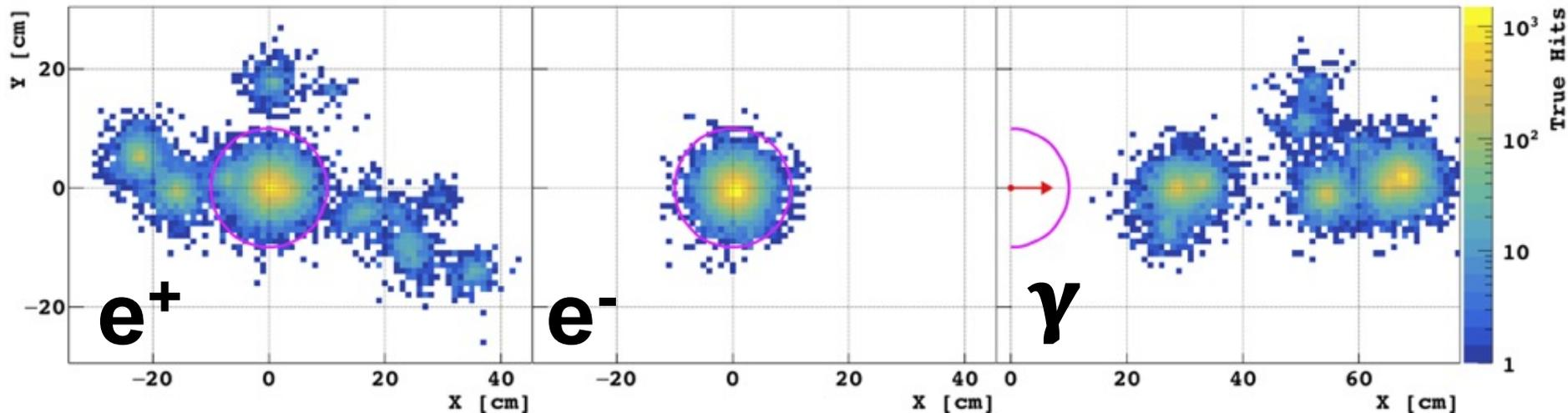
Distinguish positrons from point-like energy depositions (e.g. electrons, protons, alphas)
