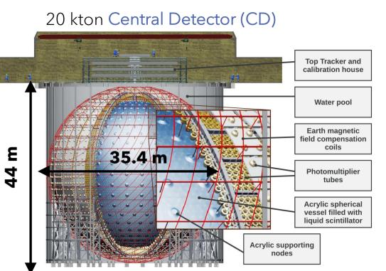
CD PMT system: 17612 20-inch (Large-)PMTs
