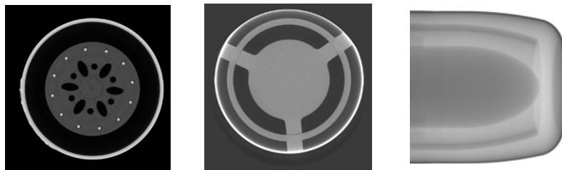
CT scans of prototype 1.3 MW target
