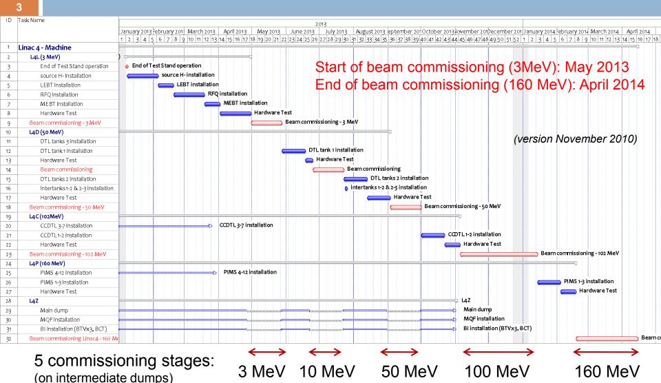
In 2013/14 (15 months), 6.5 months of beam commissioning, 3 months of HW tests, 5.5 months of installation
