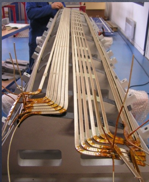
Coil winding of the Narrow and Wide circuits
