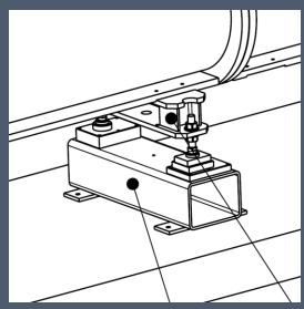
Removal of inter-section very complicated (2 more wire vacuum seals) Solution known for sections displacement only around movable feet.
