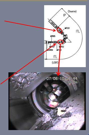
• The stripper mechanism holds 4 frames with up to 4 foils in each.
