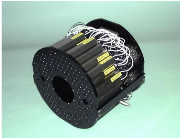
64 channels with Chrenkov radiator + PMT
