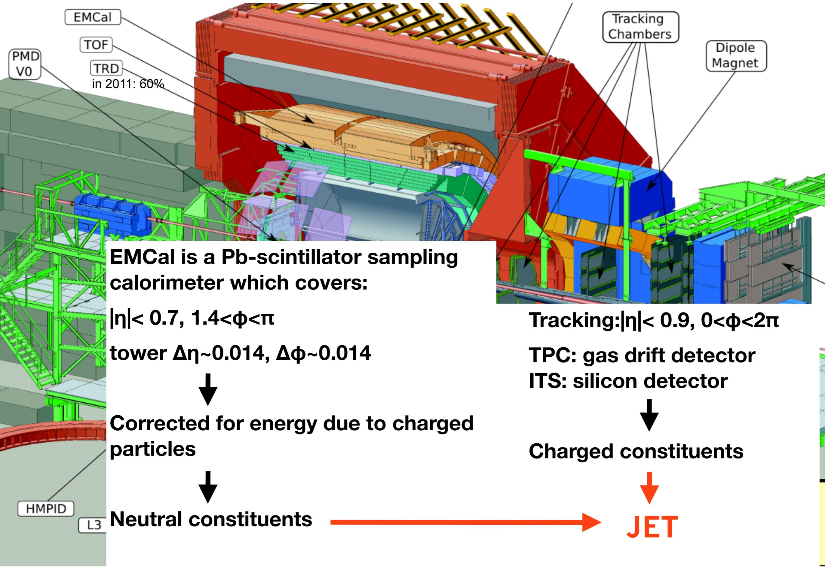
**EMCal is a Pb-scintillator sampling calorimeter which covers:**
