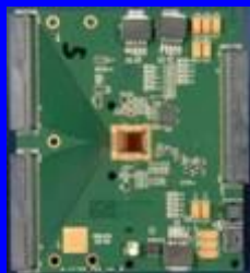
Front-end board with self-triggering n -XYTER chip
