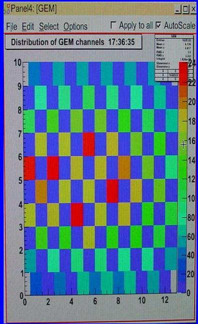
Beam spot seen on a GEM detector (every 2<sup>nd</sup> channel read out)
