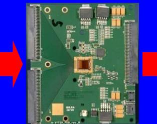
Front-end board with self-triggering *n*-XYTER chip
