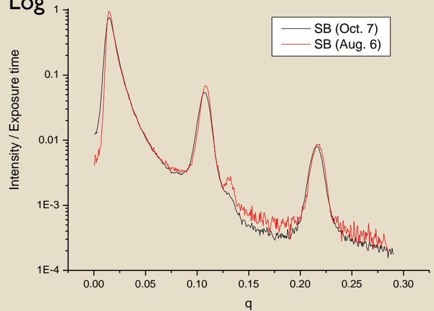
The first peaks can be different due to **beam focusing** and **fluctuation of beam flux**.
