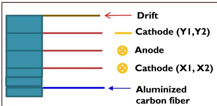
**Anode: Ø10 µm, 1.25 mm spacing.**
