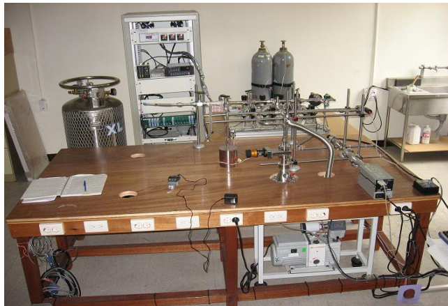
Ion pump and gas panel
