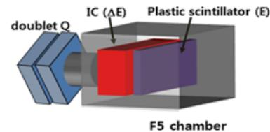
PID for low-energy recoil particle
