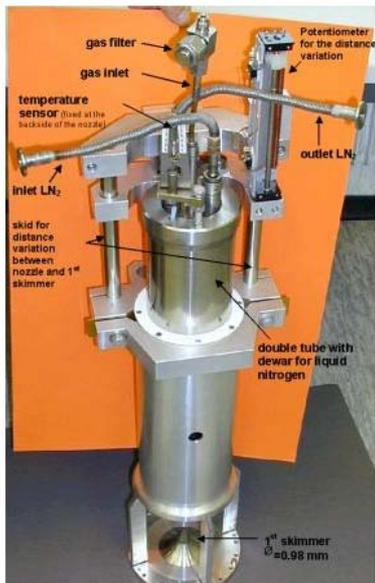
Supersonic jet gas target developed in GSI
