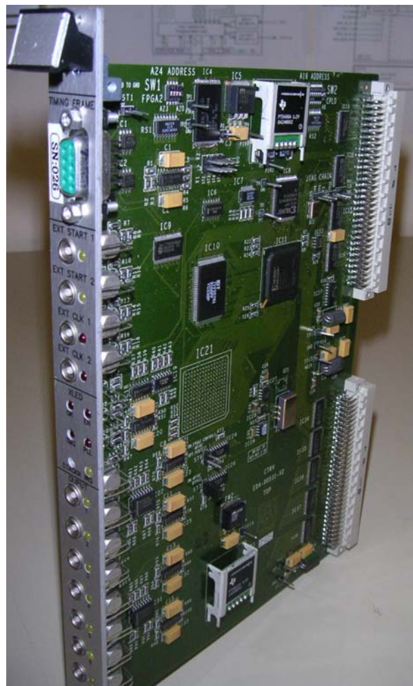
CTRV: Standard Timing Receiver card for VME systems
