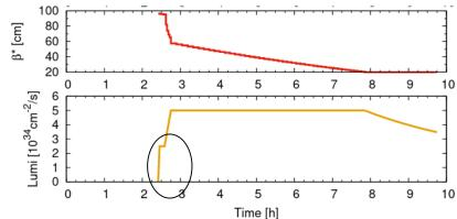
Cryo step at  $2.5 \times 10^{34}$  cm<sup>-2</sup>s<sup>-1</sup> for 10 min and then linear ramp to stabilize heat extractions. Experience could allow to reduce it.
