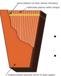
ME1/1 and ME2/1 chambers – in the most forward location, differ in material and construction
