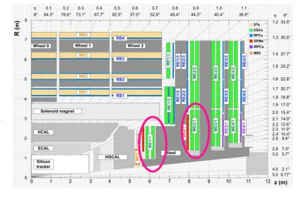
Prediction for High Luminosity LHC operation (3000 fb<sup>-1</sup>) for the most affected areas of ME1/1 and ME2/1 chambers: accumulated charge (longevity related equivalent operation time) of **0.20 and 0.13 C per cm** of anode wire
