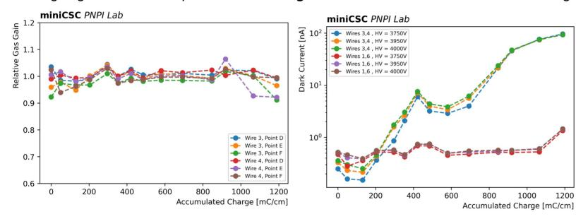
Assuming the extra-currents coming from the irradiation spot: 10 nA from ~2 cm of irradiated wire scaled to 200 m of ME2/1s1 wires give 100 uA...
