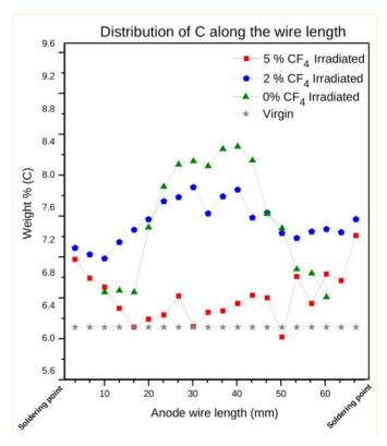
Though no miniCSC performance degradation has been seen in the longevity test – too low CF4% seems to be risky! 5%CF4 may be a good choice – also confirmed by the LHCb MUON operation experience => a longevity test with the full scale production CSCs are ongoing at GIF++ with 5%CF4
