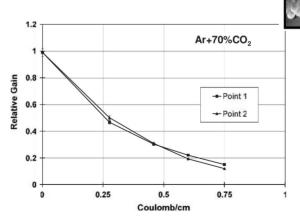
Early studies with first CSC prototypes (**Si in** contact to the gas volume - not the case in the final design) NIM A 488 (2002) 240–257
