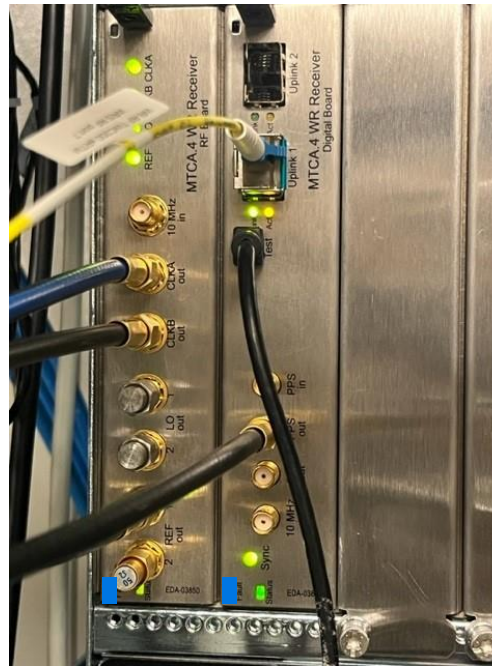
Fig – eRTM, clocks distribution
