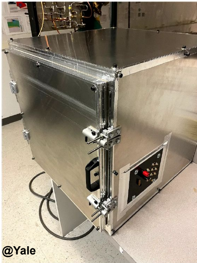
(a) Light-tight Faraday box with connector panel
