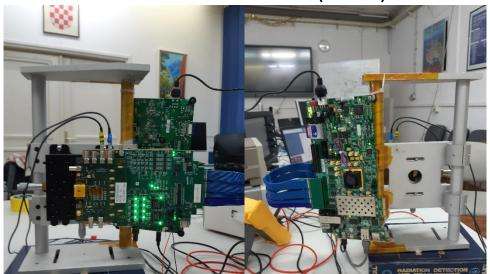
The actual DAQ toolset used for testing the MPW2 and the MPW3. It uses a ZC706 control card plus a Caribou 1.4 DAQ chipset card. The Control chip is a System On Chip Xilinx Zynq 7000 (Kyntex 7 logic fabric plus 2 ARM M9 embedded microcontrollers).
