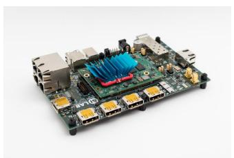
DAQ Toolset comprised of a BDAQ53 card with a Control Module inserted on top. It was designed (2016) for the RD53 hybrid detector testing (emphasis in the testing of the RD53 readout chips saga). The Control Module is an Enclustra Mercury KX2. The Mercury KX2 is a pure FPGA (Kyntex 7) from Xilinx
