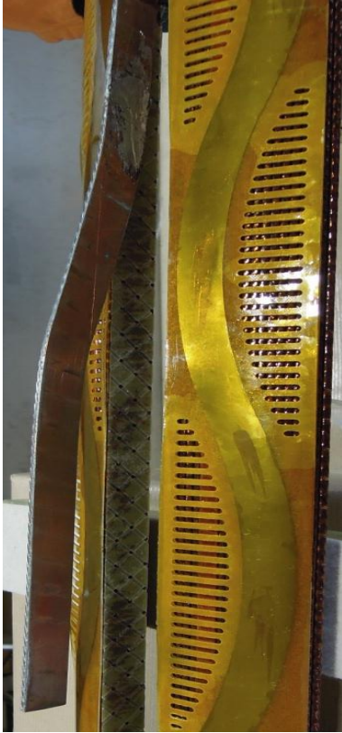
Stainless steel or SS/Cu mix Quench Heaters Long flexes up to 15m x 0.6m
