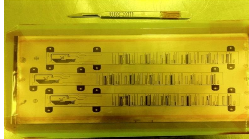
Double-sided flex for ILC Vertex sensor
