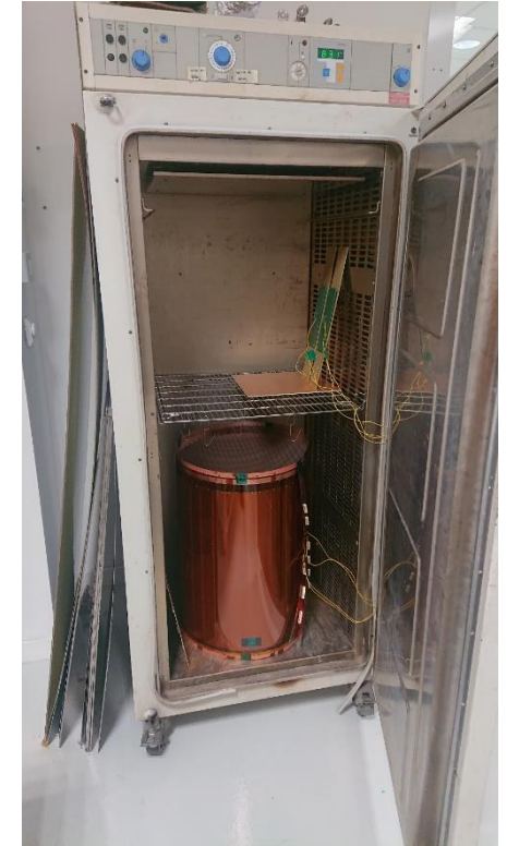
CLAS12 uRwell rolled in an oven for E-cleaning
