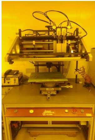
CERN precise machine 20cm x20cm deposition
