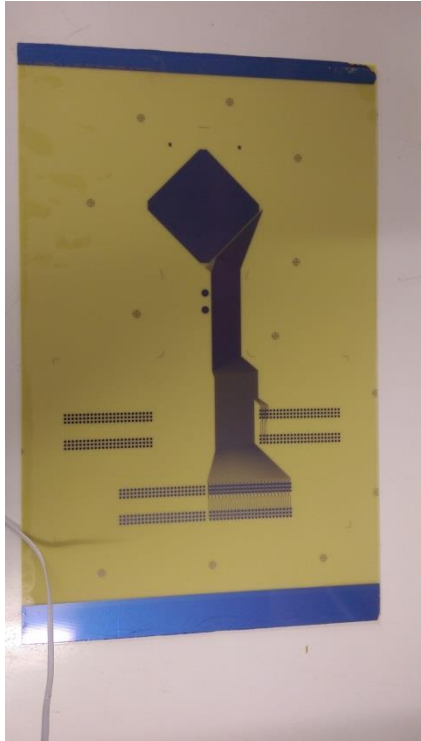
After copper Etching
