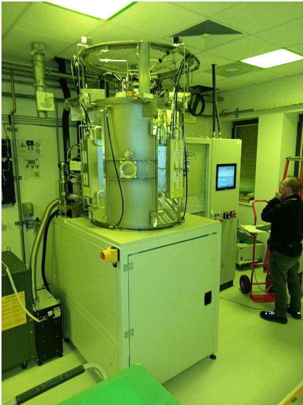
Pulsed DC Magnetron vacuum deposition machine
