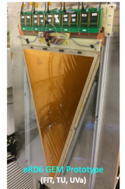
CORE EIC GEM prototype U-V strip readout
