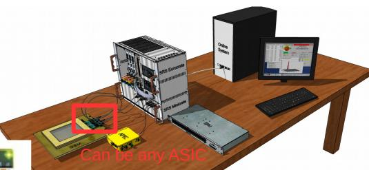
Implementation of ASIC in SRS requires: Hybrid, adapter card, FEC FPGA firmware
