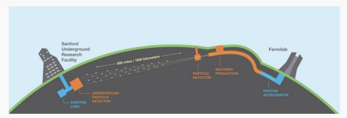
The Deep Underground Neutrino Experiment (DUNE) is a next-generation international experiment for neutrino science. DUNE will consist of two sets of neutrino detectors placed in the LBNF beamline. The near detector (ND) will observe the beam near its origination, 1 km underground at Fermilab in Batavia, IL. The larger far detector (FD) will be installed 1.5km underground, 1,285 kilometers away, at the Sanford Underground Research Facility (SURF) in Lead, South Dakota.
