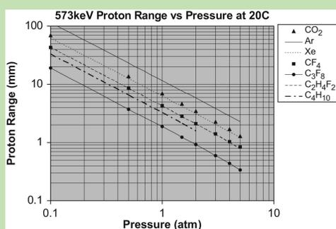
Figure 2. Ranges of protons calculated from SRIM simulations in various stopping gases at increasing pressures [3].
