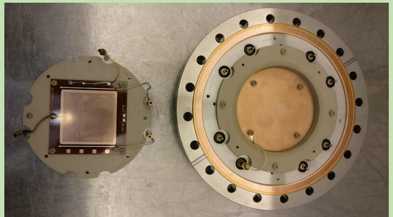
Figure 5. The  $\mu$ RWELL shown alongside the copper plate used as a drift electrode, before the pressure vessel was closed.
