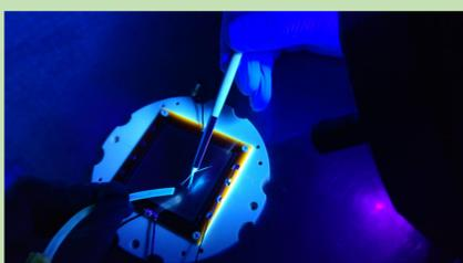
Figure 4. Removing dust particles located with a UV light.
