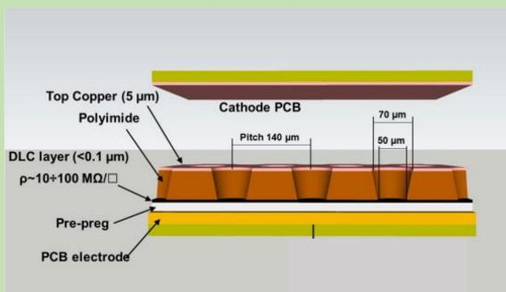
Figure 1. Layout of the  $\mu$ RWELL [2].
