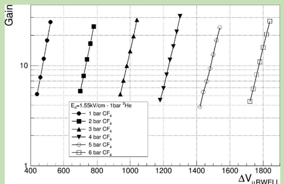
Figure 6. Gain curves from 1 bar to 6 bar of  $\text{CF}_4$ , shown with the corresponding voltage applied across the  $\mu$ RWELL.
