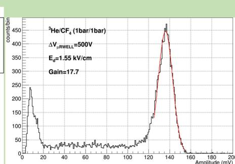
Figure 3. Pulse height spectrum from a neutron interaction within helium-3.
