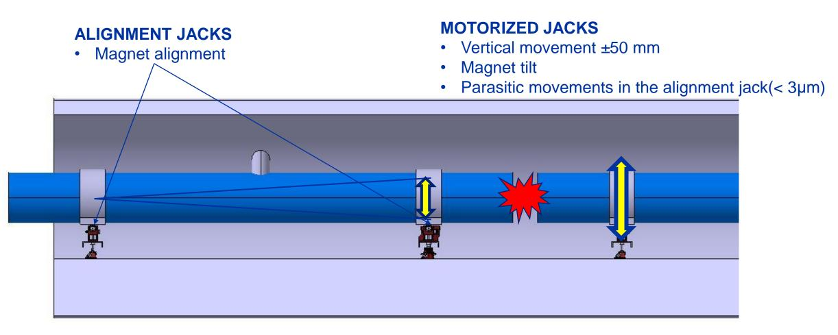
Maximum stroke in opposite direction over the interconnection will destroy the bellows! SAFE OPERATION SHALL NOT RELY ON THE CONTROL SYSTEM!
