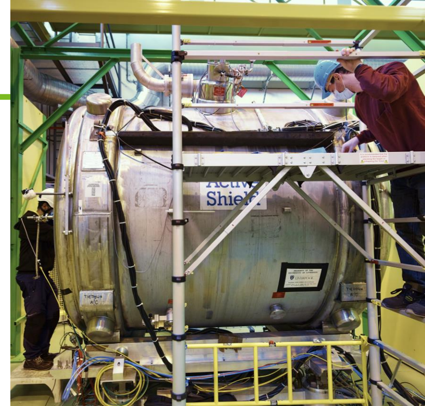
4T superconducting (former MRI) solenoid from UQ hospital, Brisbane to ISOLDE in 2017
