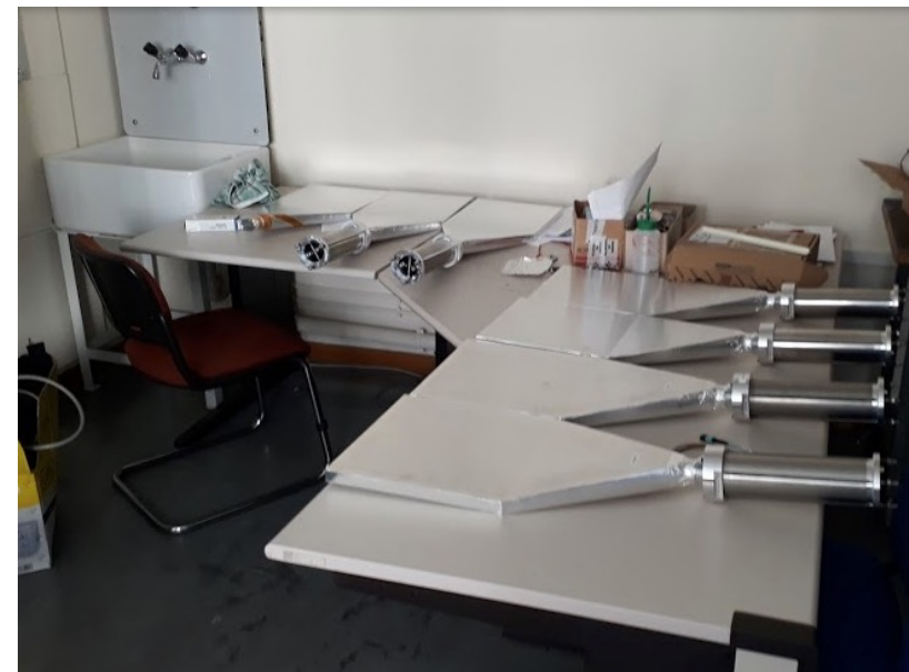
Scintillators, light guides and PMT housing constructed at CERN scintillator lab (EP-DT).
