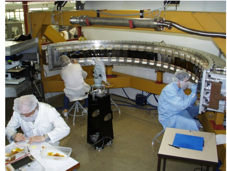
Telescope of 32 MSGCs tested at PSI in Nov99 (CMS Milestone)
