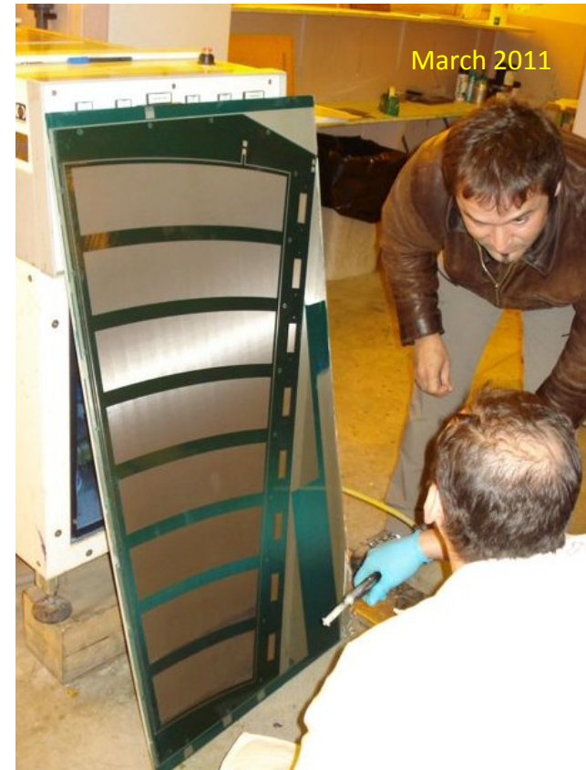
1.2 x 0.6 m 2 prototype chamber with 2048 readout strips (0.5 mm strip pitch) during construction in CERN/TE-MPE workshop
