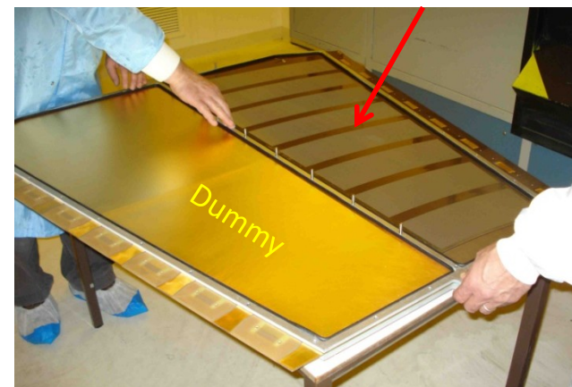
0.6 x 1.2 m 2 MicroMegas with resistive-strip protection
