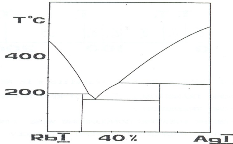
Figure 3. Phase diagram of RbI + AgI system (Ref. 2). Deep eutectic near the molar ratio 4 : 1. If the temperature is more than 228^{\circ}\text{C} (melting point of \text{RbAg}_4\text{I}_5 ) - the system 25% RbI + 75% AgI is the melt, if the temperature is less - the system became the crystal \text{RbAg}_4\text{I}_5 .
