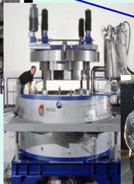
Varian (2005) 90 Tons Isochronous Cyclotron
