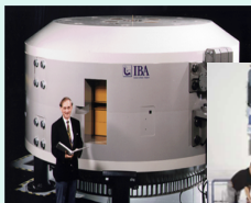
IBA (1996) , SHI 250 Tons Isochronous Cyclotron
