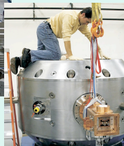
MEVION (2013) 15 Tons Synchrocyclotron
